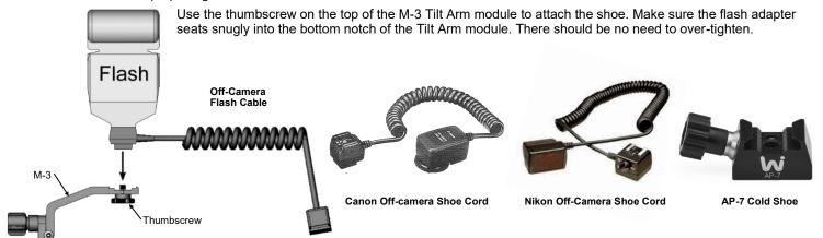
The AP-7 cold shoe adapter can be used to mount the Speedlight flash unit to the flash bracket's mounting stud. The Nikon AS-20 can also be used. Contact us if you have trouble mounting your flash to the bracket.
