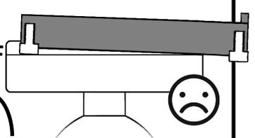
Clamps without safety stop channels (or those without adequate clearance) will **insecurely** clamp the foot at an angle
