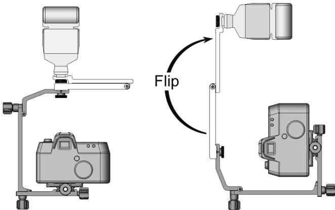
The M-7 module is a useful accessory for both wedding and portrait photography. The elevation of the flash unit above the camera body reduces both red-eye and distracting, unflattering shadows when photographing people.
