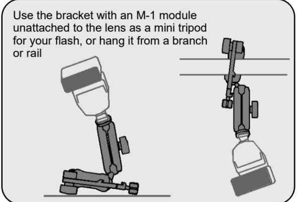
Use the bracket with an M-1 module unattached to the lens as a mini tripod for your flash, or hang it from a branch or rail
