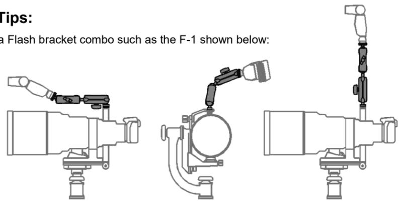
After extended use you may have trouble with the balls slipping or creeping when fully tightened. If this occurs try washing the rubber surfaces with a small amount of dishwashing soap and a toothbrush to remove any oils that may have gotten onto the rubber. Rinse well and allow to dry thoroughly before using.
