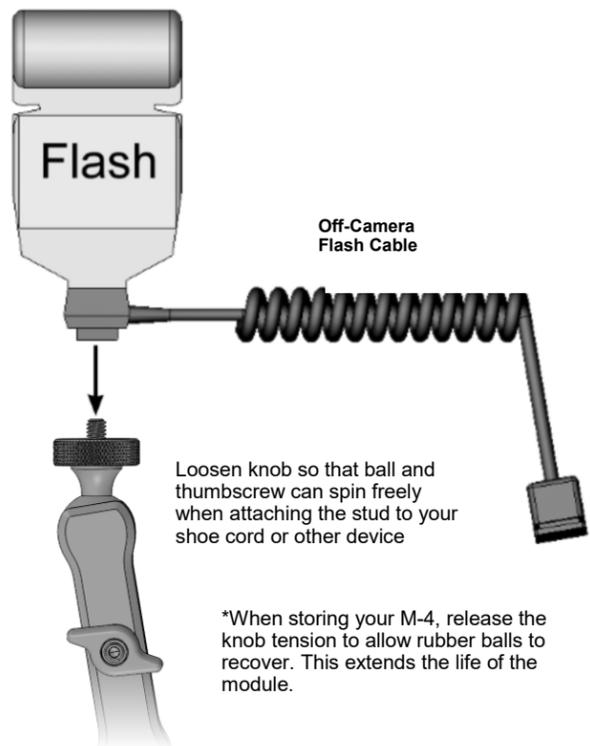
Loosen knob so that ball and thumbscrew can spin freely when attaching the stud to your shoe cord or other device
