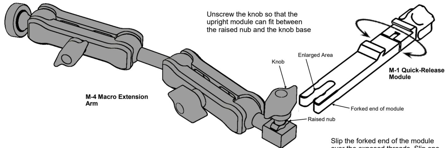
Unscrew the knob so that the upright module can fit between the raised nub and the knob base
